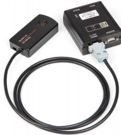
Connecting the GyroSet™ Link to IOM
