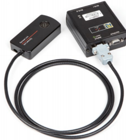
Connecting the GyroSet™ Link to IOM
